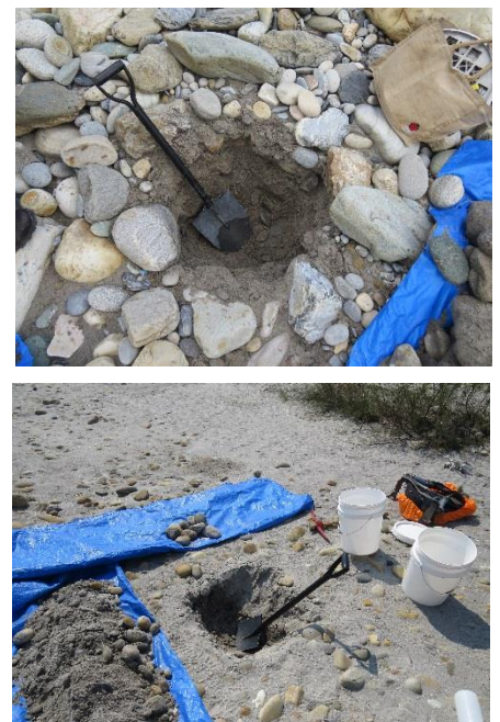
Figure 1 Subsurface grain size measuring. Step 1 – dig a huge hole!
