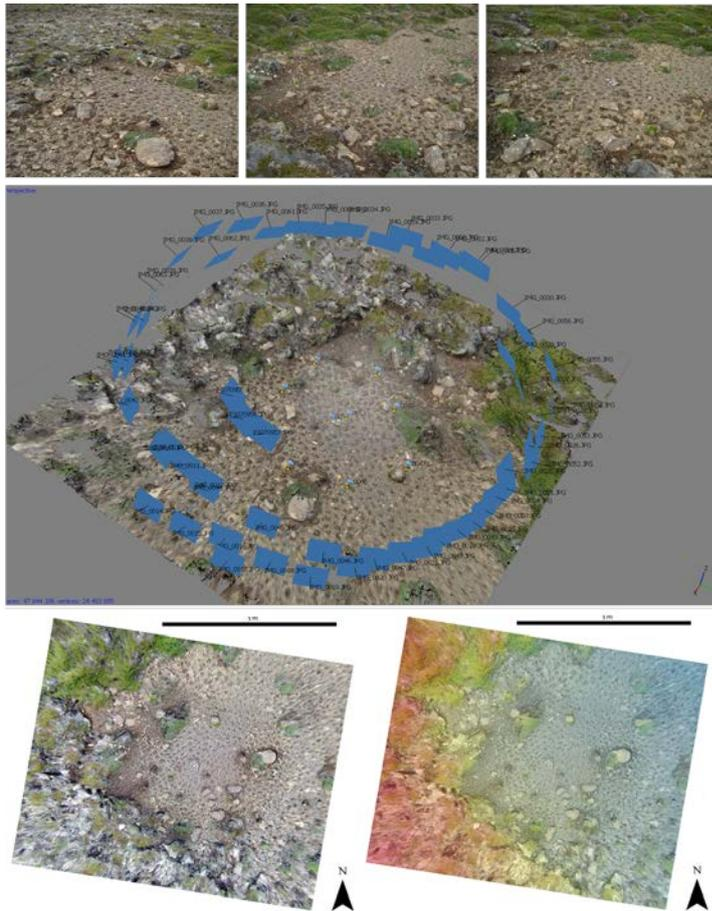
***Building a 3D model using Structure from Motion, Photographs are taken from multiple angles and then points within them are matched to create a model of the site.***
