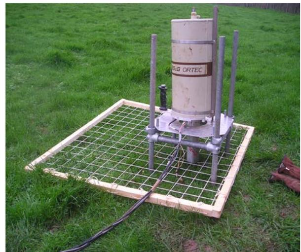
Figure 1. Using an *in-situ* gamma spectrometer to measure areal activity.
