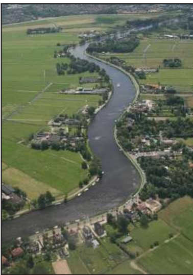
Figure 12. Oblique aerial view of a typical sinuous river within a wide, cultivated and settled floodplain in western Europe. Although the sinuous planform gives the impression of active meanders, the river is now constrained by bank protection works and no meandering now takes place (Photo: Stephen Tooth).
