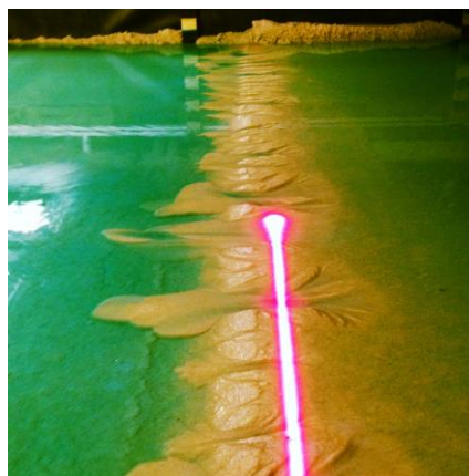
Figure 1 – A topographic laser scan captures mm-scale experimental washover topography during laboratory trials at the National Center for Earth-surface Dynamics, St Anthony Falls Laboratory (University of Minnesota, USA).
