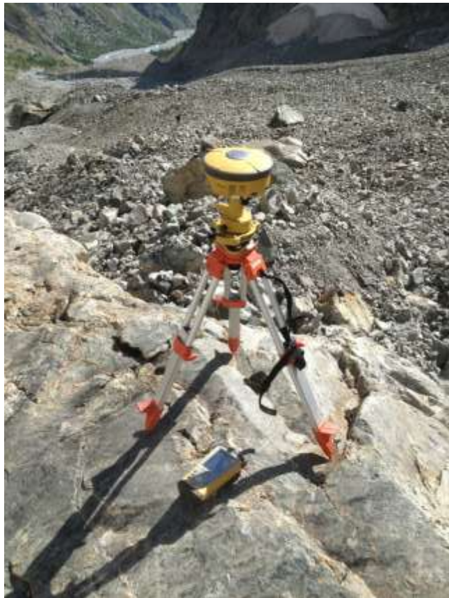
Figure 7: The base station for dGNSS measurements was installed on the top of house-size boulder
