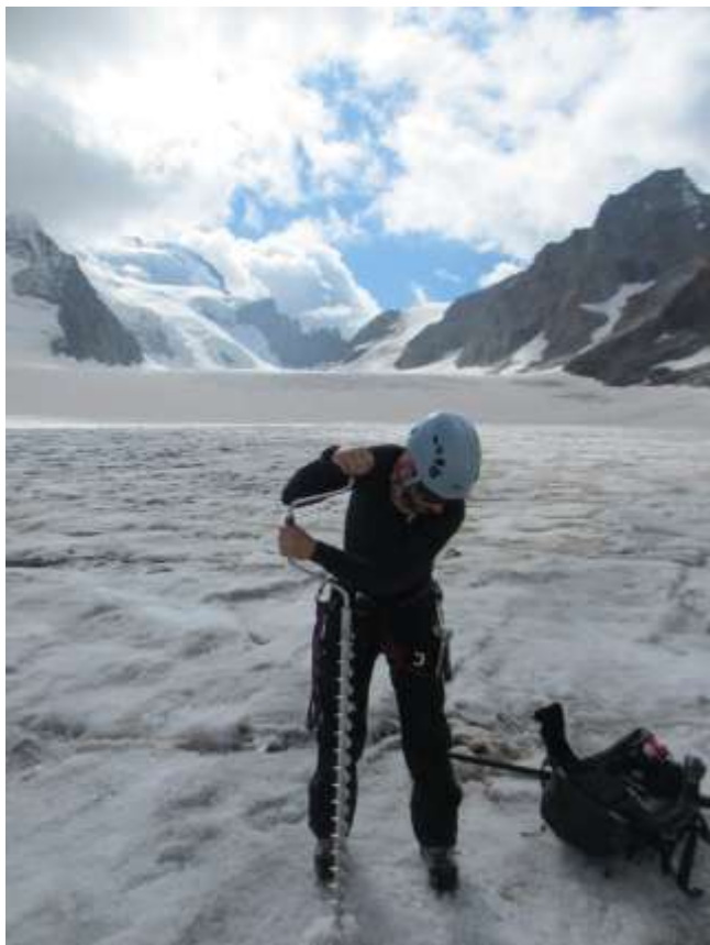
Figure 5: Hand drilling for ablation stakes on Glacier Blanc
