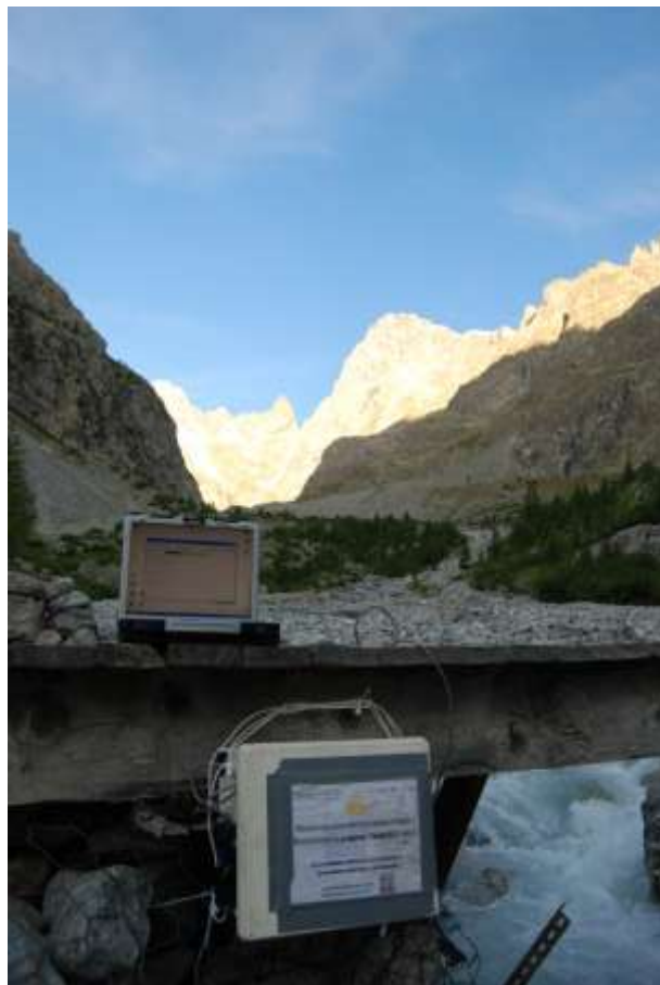
Figure 9: The water gauging station was set up under the bridge of Glacier Noir Stream
