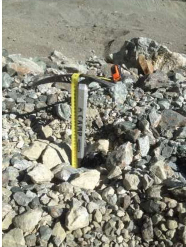
Figure 4: Debris thickness measurement
