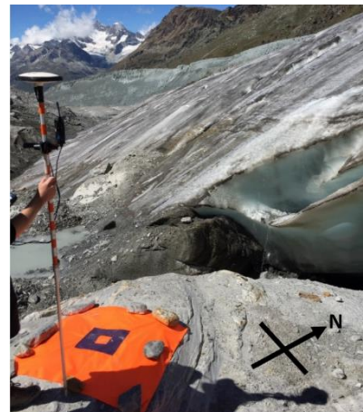
Figure 1. Example of GCP with DGPS to accurately georeference.
