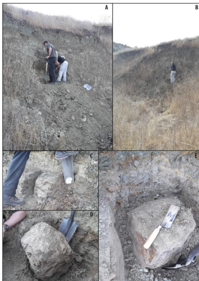
Figure 2. Collection of undisturbed blocks of sediment from the Hollister Hills State Vehicular Recreation Area, California, USA. A and B display the sampling locations within the slope. C, D and E display the gradual isolation and removal of the undisturbed blocks.
