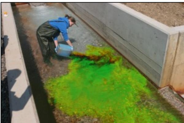
Figure 5. Photograph showing injection of a fluorescent tracer into a channel (courtesy: [http://www.openchannelflow.com/blog/archives\\_article](http://www.openchannelflow.com/blog/archives_article)).
